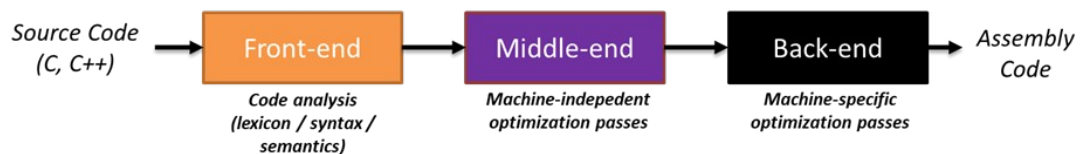
Figure 32: Main blocks composing a standard compiler toolchain
